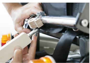
Put the joint head on top of the trailer over the screw and connect it to the HITCH by unscrewing the wing bolt. Tighten the wing bolt firmly by hand.
