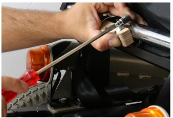
Tighten the screws of the pipe clamps. You also have to check these screws regularly.
