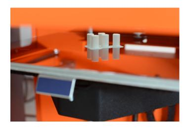
We could produce wooden dowels of 8 mm diameter and 14 mm length.
