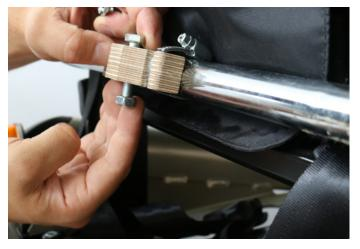
Insert the hex bolts into the holes and screw the nut tightly.
