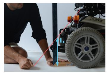
Mark first the middle line of the pipe. Attach a string to the marked line and use an adhesive tape to prevent it from slipping. Run the line collision test and attach the obstacle.
