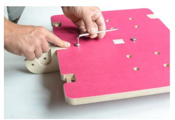
Insert screws into the two holes located in the center of BOARD and tighten them.
