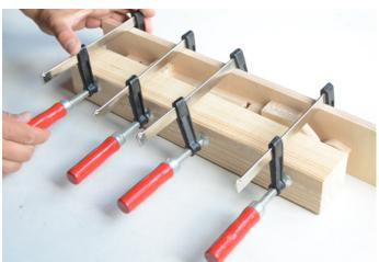
Press the parts together with 2 stable supports and several screw clamps.
